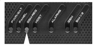
4. The 'GSM REG' LED will also indicate whether the modem is operational or experiencing any issues. Green flashing = Currently registering on the GSM network.
