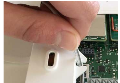
Insert the wire into the strain-relief
