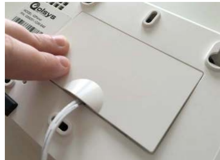
Push the cover down until it snaps in place
