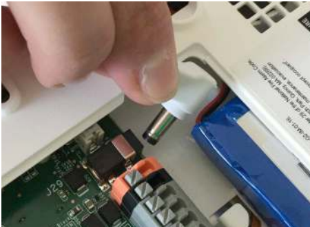
Plug in the power connector
