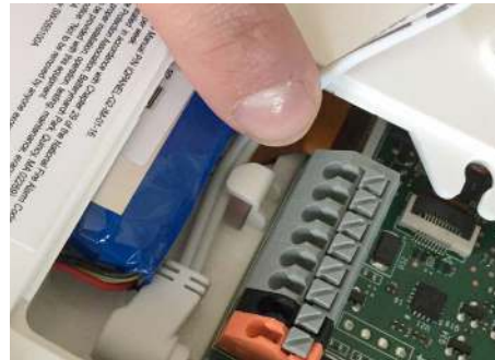
Route the wire behind the retainer clip
