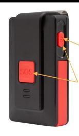
When off, press and hold for 3 seconds to turn the device on.
